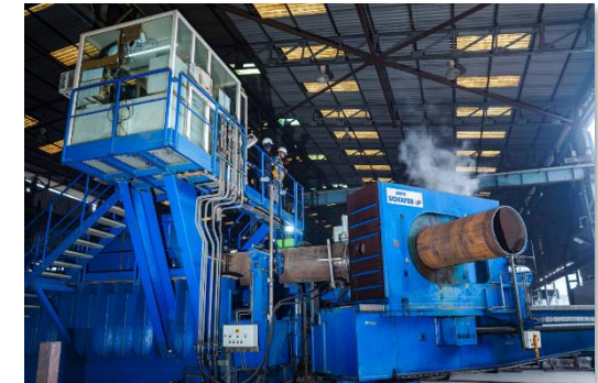
Induction bending process
