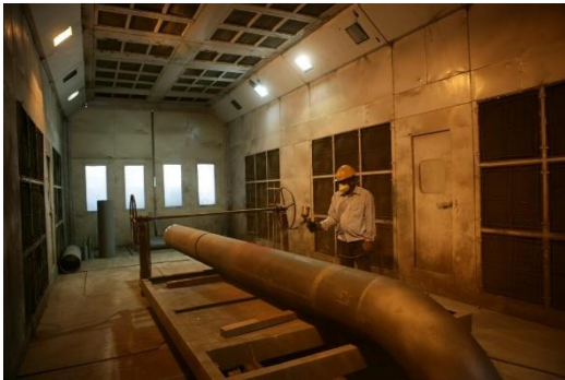
Semi-automatic shot blasting and painting machines
